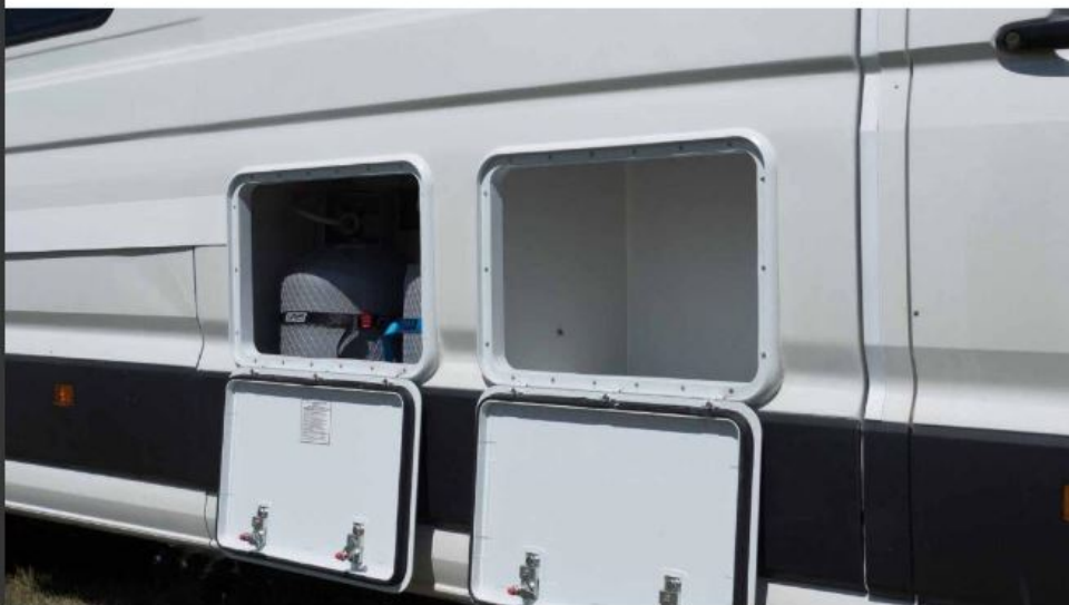
Two lockers in the slide-out house the gas cylinders and provide good room for hoses, power leads and the like. There's a third locker on the kerb-side for storage or optional generator.
